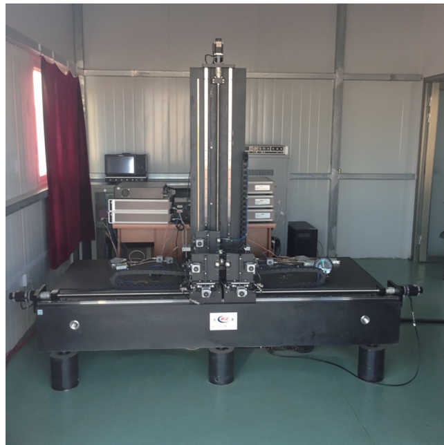
图5 移动式T型发射架 Fig. 5 Picture of T shape transmitter array with moving aperture
