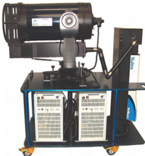
图6 美国陆军实验室与 Applied Photonics 公司合作开发的双脉冲 LIBS 系统 [39] Fig.6 DP-LIBS system developed by ARL and Applied Photonics, Ltd. [39]
