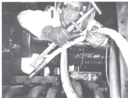
图3 用于反应堆探测的光纤 LIBS 探头 [18] Fig.3 Optical fiber LIBS probe for reactor detection [18]
