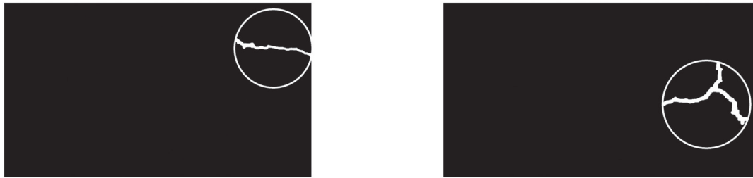
(a) The smallest circumscribed circle of single-line cracks ( R=243 ) (b) The smallest circumscribed circle with bifurcation cracks ( R=272 )
