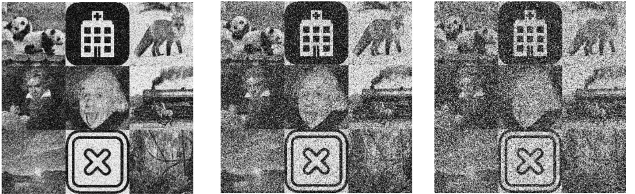
(a) Decrypted image with \sigma=0.1 Gaussian noise (b) Decrypted image with \sigma=0.3 Gaussian noise (c) Decrypted image with \sigma=0.5 Gaussian noise
