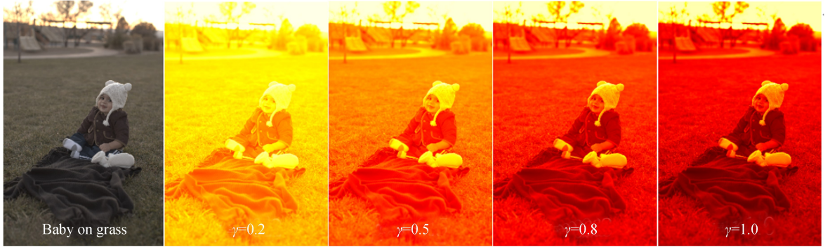
(c) Input low-light images and illumination map calculated with different \gamma values
