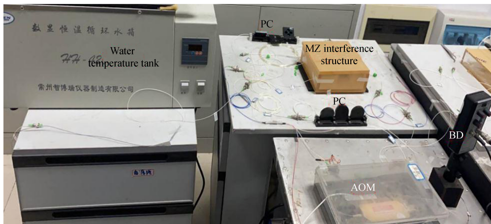
图6 复合频移干涉温度传感系统 Fig.6 MFSI temperature sensing system
