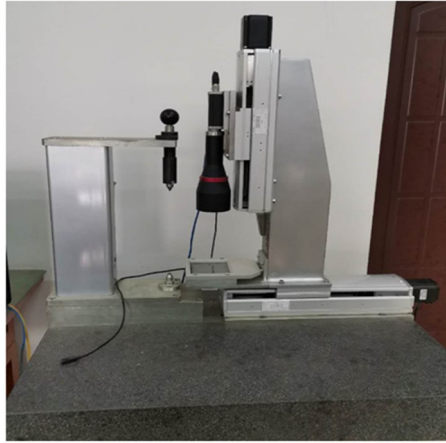
图5 齿轮视觉测量装置结构 Fig. 5 Structure of gear vision measuring device
