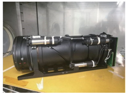
图 7 三十倍连续变焦系统完成高低温试验 Fig.7 Temperature test of 30× continuous zoom lens
