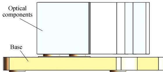
图3 光学组件粘接示意图 Fig.3 Adhesive schematic diagram of optical components
