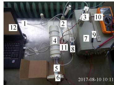
1. Gas inlet (from pump); 2. Formaldehyde bottle; 3. Inlet sensor; 4. Photocatalytic filter reactor; 5. Fiber bundle; 6. Ultraviolet LED; 7. Constant current power supply; 8. Outlet sensor; 9. Phototube; 10. AVOmeter; 11. USB hubs; 12. Computer
