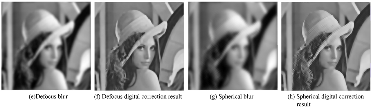
图3 彗差、像散、离焦、球差校正前后图像对比 Fig.3 Comparison of four kinds of aberration's digital correction results
