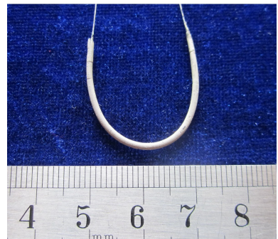
图5 保护后 U 型弯曲光纤 Fig.5 The U-shaped fiber with the inner India ink layer and outer nickel coating
