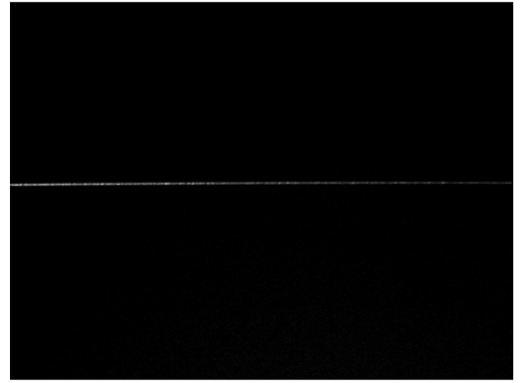
图3 CCD 侧向散射激光雷达回波信号图 Fig.3 The echo signal diagram based on the CCD side-scattering lidar
