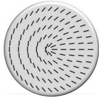
图 1 Pancharatnam-Berry 相位元件的光轴(慢轴)分布示意图 Fig.1 The optical axis (slow axis) spatial distribution of the Pancharatnam-Berry phase element
