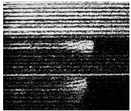
图 9 双轴 VISAR 获得的有条纹移动的实验图像 Fig. 9 Interferogram with fringe moving obtained by two-axis VISAR
