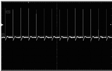
图6 泵浦功率为 3.5 W 时,五个波长连续锁模波形图 Fig. 6 Harmonic mode locking waveform with pump power of 3.5 W
