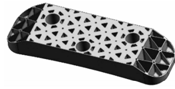
图 1 初始的轻量化反射镜结构 Fig. 1 Original structure of lightweight reflective mirror
