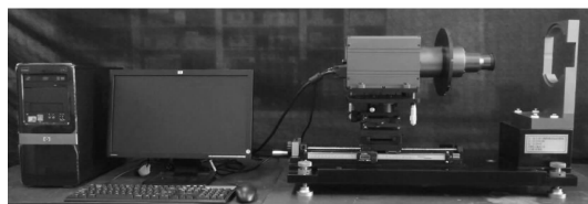
图 1 LCoS 拼接动态星模拟器实物照片 Fig. 1 The photo of LCoS splicing dynamic star simulator
