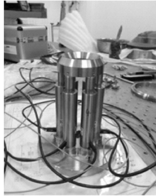
(b) Assembled actuate ring and six actuators
