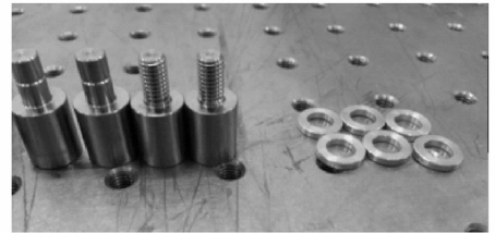
(b) Connector between actuator and actuate ring
