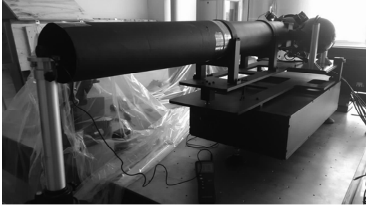
Fig. 7 Test system for star simulator
