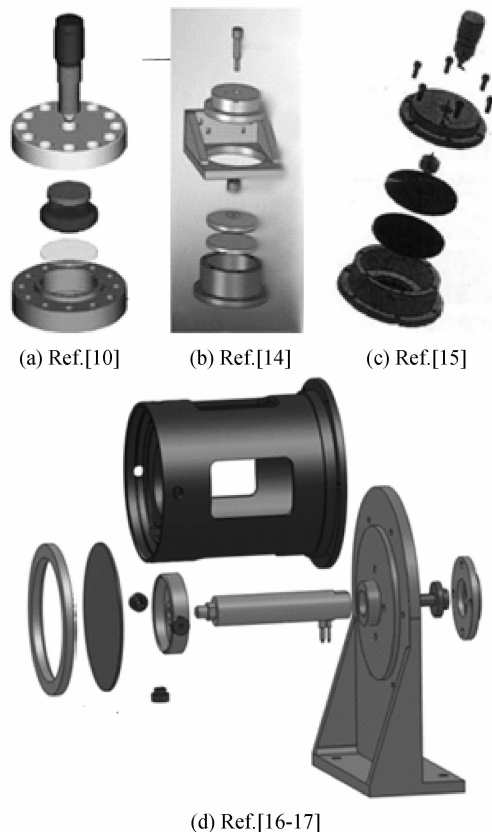
图1 参考文献[10, 14-17]中设计的变曲率反射镜结构 Fig. 1 Annular force based prototype variable curvature mirror designed in literatures [10, 14-17]
