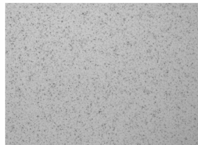
(b) Optical microscope test result(500×) of 50nm/5nm Pt/Cr sample
