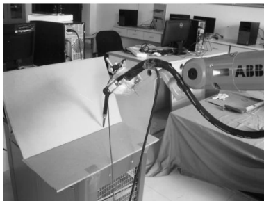
图 5 机器人沿平板交线运动 Fig. 5 The robot motion along the flat intersection
