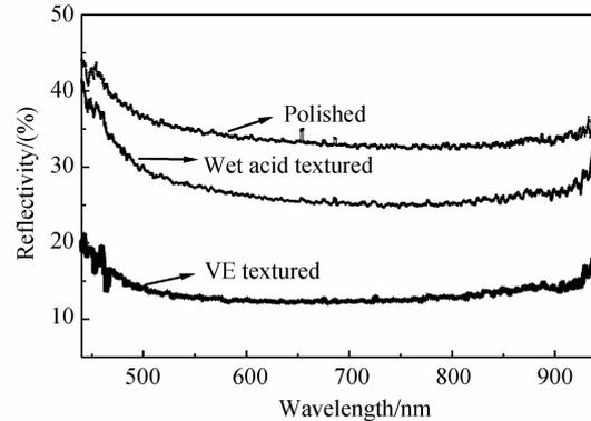
Fig. 3 Reflectivity of polished silicon wafer, silicon wafer with VE textured, and silicon wafer with wet acid textured
