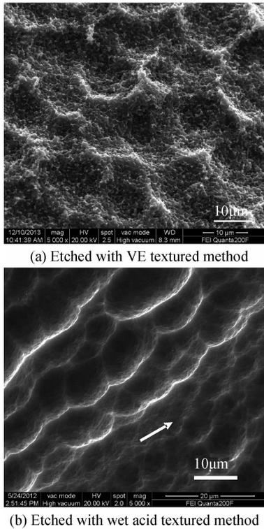
Fig. 2 SEM micrographs of wafers
