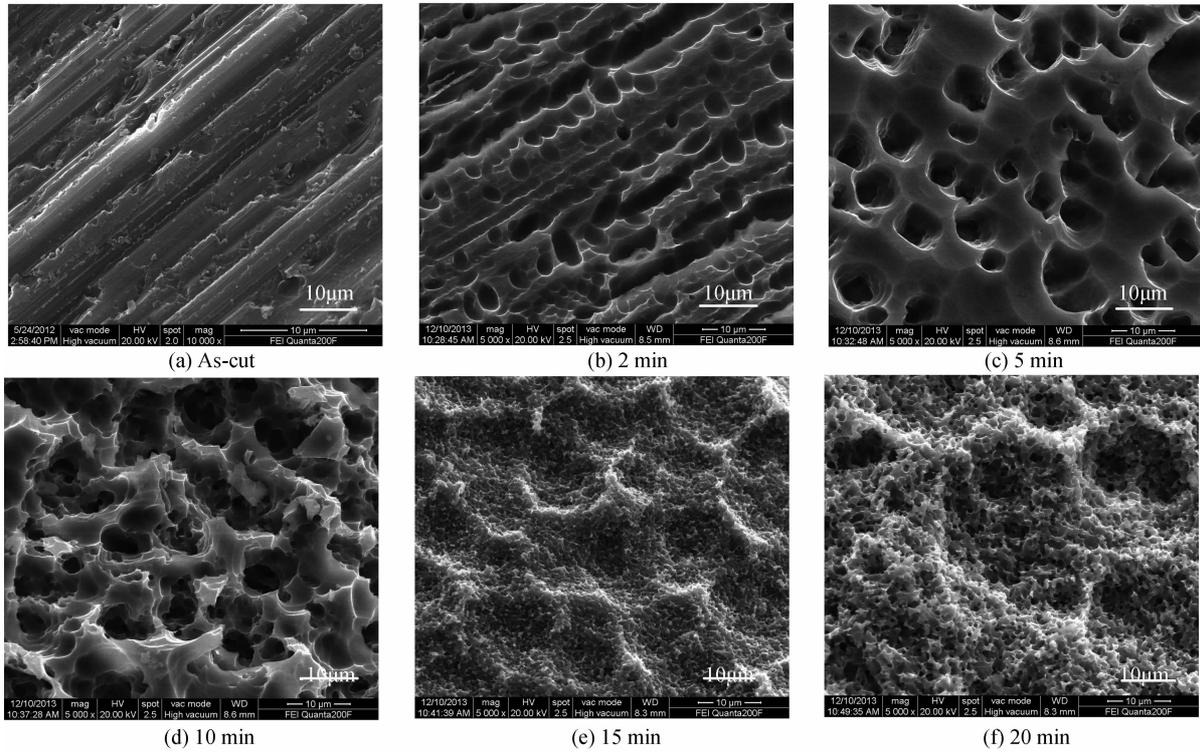
Fig. 5 Evolution of micrographs of DWS mc-silicon wafers etched in vapor (SEM)
