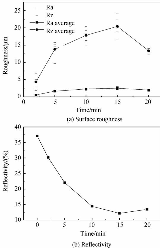
Fig. 6 The surface roughness and reflectivity curves of silicon wafer with different etching time
