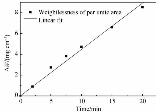
Fig. 4 Weight loss of dissolved silicon wafers versus the etching time
