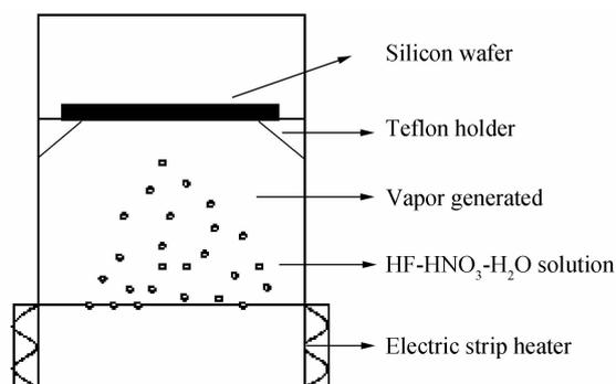
Fig. 1 Schematic representation of the vapor texturing setup
