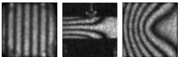
图5 无阈值窗口傅里叶滤波滤波后的图样 Fig. 5 Filtered fringe pattern by non-threshold windowed Fourier filter
