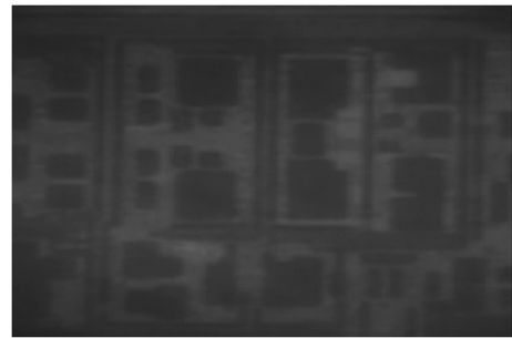
图 7 50\times 显微物镜激光红外显微成 SRAM 器件灵敏区的图像 Fig. 7 SRAM devices sensitive region image by microscope infrared imaging technology with 50\times microscope objective
