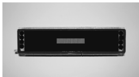
Fig. 4 Real photograph of integral type cold cathode FED prototype
