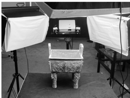
Fig. 2 Experiment setup for digitizing movable cultural heritage
