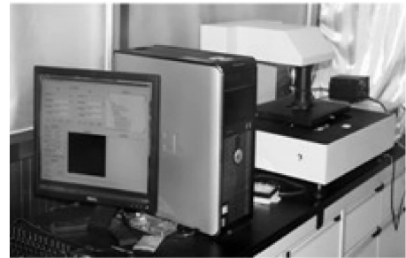
图5 计算全息图直写打印系统 Fig.5 The system of computer-generated hologram printer
