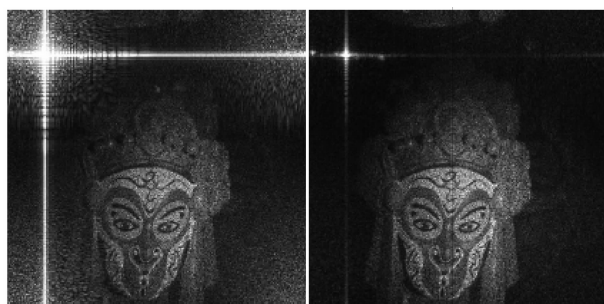
(a) Synthesized image with zero-order M=0.15 (b) Synthesized image with zero-order eliminated M=0.15
