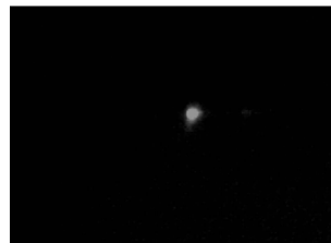
图 7 M-Z 型波导近场输出光斑 Fig. 7 Output near-field spot of M-Z waveguide
