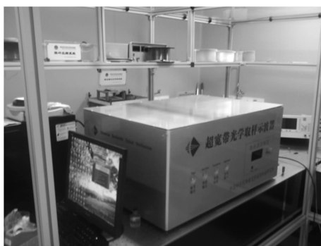
图 11 研制出的超宽带全光取样示波器实验样机系统照片 Fig. 11 Photograph of the developed ultra-wide bandwidth all-optical sampling oscilloscope prototype system
