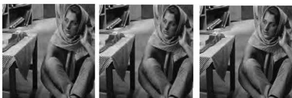
(a) SPIHT, 0.125bpp, 24.86dB, (b) JPEG-2000, 0.125bpp, 25.24dB, (c) Proposed algorithm, 0.125bpp, 27.95dB
