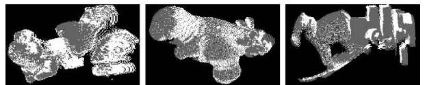
(b) Recognition model images overlaid on the test objects with the recovered pose
