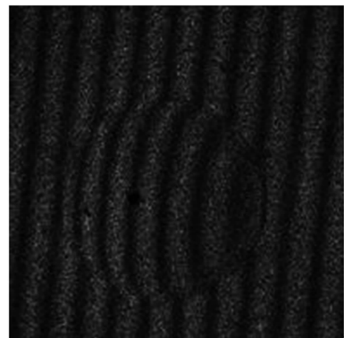
图 3 偏转物面引入的干涉条纹 Fig. 3 Interference fringe pattern introduced by tilting object
