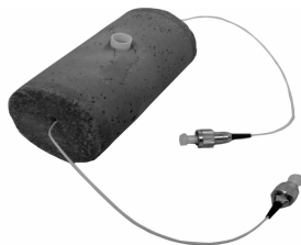
图8 镀膜光纤埋入混凝土试块 Fig.8 Concrete block with metallized fiber in it
