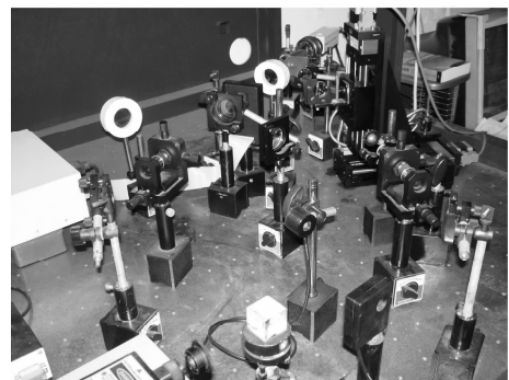
图 4 体全息存储光路系统平台 Fig. 4 Experimental equipment of optical holographic storage system
