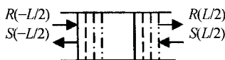
图 1 多波长啁啾叠栅的矩阵分析模型 Fig. 1 Model of superimposed multi-wavelength CFBG for Matrix analysis
