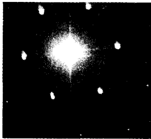
图 4 硅(111)面衍射谱 Fig. 4 Diffraction spectrum of a TEM image of Si(111)
