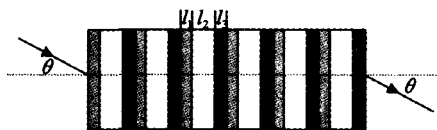
Fig. 1 Schematic structure of 1D polybasic photonic crystals consist of alternative layers of three kind of materials. By introducing structural parameter a and b , 1D ternary periodic photonic crystal with m periods and center wavelength \lambda_0 can be defined as
