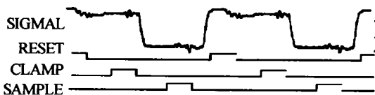
图4 未采样信号与复位、钳位、采样信号对比 Fig. 4 Signal unsampled of one pixel and RESET, CLAMP, SAMPLE
