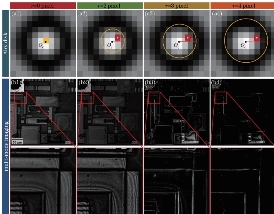
图 13 设计不同的数字针孔重建各向同性的多模式图像。(a1)设计数字针孔抽取共轭物点发出的零频信号;(a2)~(a4)设计偏置的数字针孔从不同方向抽取非共轭物点发出的高阶衍射信号;(b1)~(b4)利用从不同方向抽取的信号重建的各向同性的多模式图像 Fig. 13 Reconstruction of isotropic multimodal images using differently designed digital pinholes. (a1) Design digital pinhole to extract the zero-order signal from the conjugated object point; (a2)~(a4) design offset pinholes to extract high-order diffraction signals from non-conjugated object points in different directions; (b1)~(b4) isotropic multimodal images reconstructed using signals extracted from different directions
