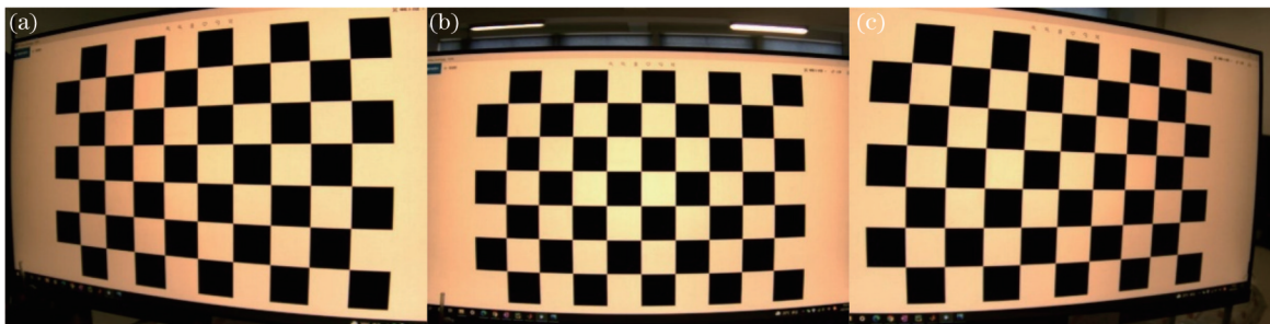
图5 棋盘格靶标原始图像。(a)图像1;(b)图像2;(c)图像3 Fig. 5 Original images of checkerboard targets. (a) Image 1; (b) image 2; (c) image 3
