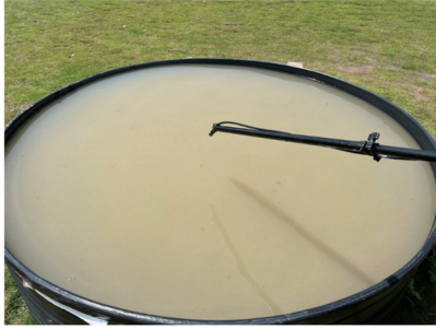
Fig. 2 Photo of the water-filled tank along with the radiometer when taking measurement of L_t via above-water approach (AWA)
