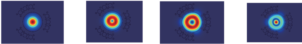
图 3 密集空气孔辅助的 4-LP 少模光纤模式图 Fig. 3 Mode diagram of 4-LP few mode fiber assisted by dense air holes
