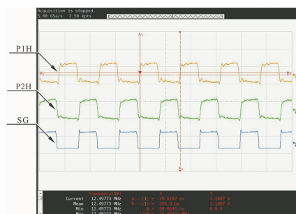
图 5 探测器驱动信号的波形 Fig. 5 Waveform of detector drive signal
