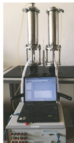
图 10 双光纤光栅静力水准仪的标定实验 Fig. 10 Calibration test of double fiber Bragg grating static level
