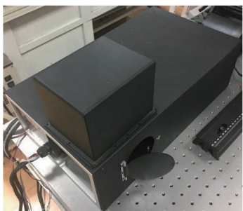
图 7 像场调制傅里叶变换成像光谱仪样机 Fig. 7 Prototype of image field modulated Fourier transform imaging spectrometer
