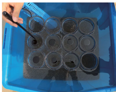
图1 实验模拟的海洋环境以及不同厚度海面溢油油膜 Fig. 1 Simulated marine environment and sea-surface spilled oil with different thicknesses
