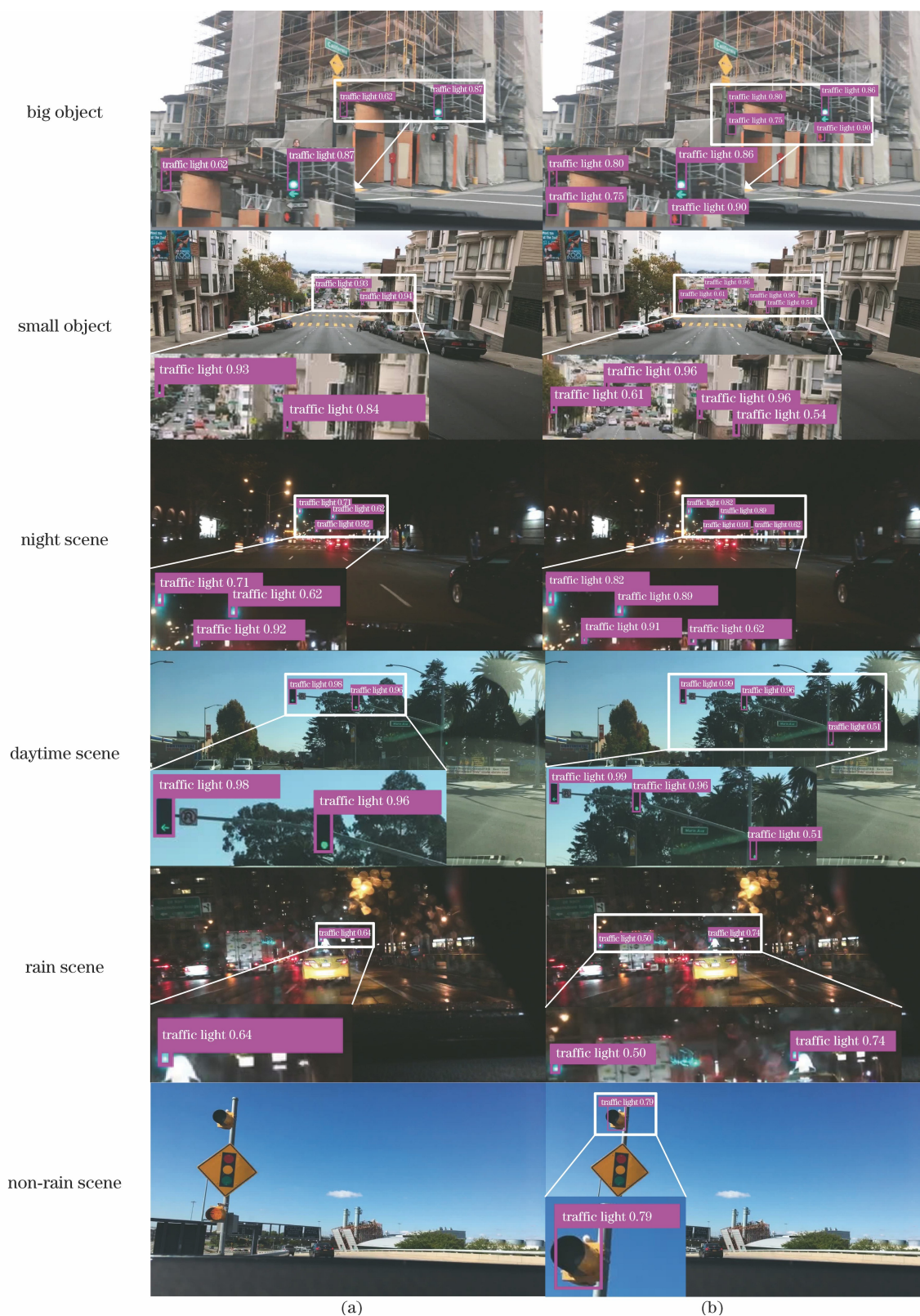
图 11 检测结果对比。(a) YOLOv3 算法检测结果;(b) YOLOv3 优化算法检测结果 Fig. 11 Comparison of detection results. (a) Detection results of YOLOv3 algorithm; (b) detection results of optimized YOLOv3 algorithm
